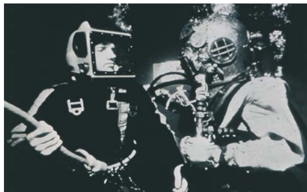
Fig. 31-7. US Navy Mark (Mk) 12 (left) and Mk V (right) diving helmets. The Mk V was used until 1980, when it was replaced by the Mk 12. The Mk 21 replaced the Mk 12 in 1993. Reprinted from US Department of the Navy. US Navy Diving Manual . SS521-Ag-PRO-010. Washington, DC: Naval Sea Systems Command. Rev 4 (20 Jan 1999); Change A (1 Mar 2001): p1-9. NAVSEA 0994-LP-100-3199.
